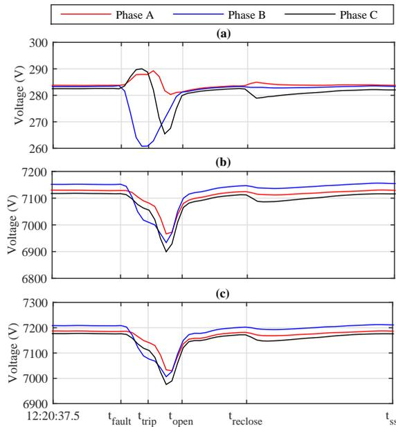
Fig. 10. Synchronized voltage magnitude measurements during fault in three outlying locations: (a) Micro-PMU 3, (b) Micro-PMU 4, (c) Micro PMU 5.
