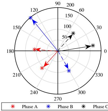
Fig. 7. Three-phase current phase angle and magnitude fluctuation of Micro-PMU 2 during fault: dash-line at  $t_{\text{fault}}$  and solid-line at  $t_{\text{trip}}$ .
