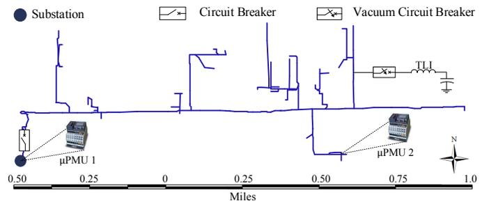
Fig. 1. Test system is a real-life feeder in Riverside, CA, which includes a switched capacitor bank and is equipped with two  $\mu$ PMUs.
