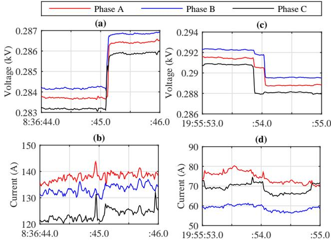
Fig. 7. Load level dynamic response to capacitor switching event: (a) Voltage transient at *switch on* event, (b) Current transient at *switch on* event, (c) Voltage magnitude at *switch off* event, (d) Current magnitude at *switch off* event.
