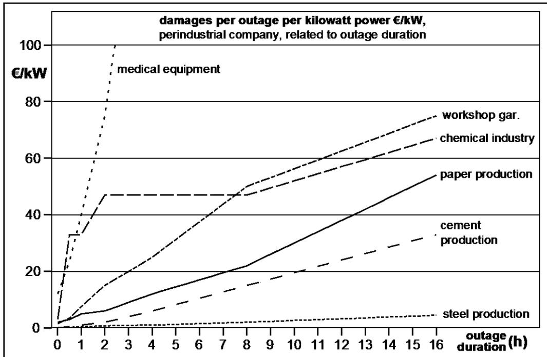
Figure 4 – Interruption costs as a function of outage duration, KEMA 2005.
