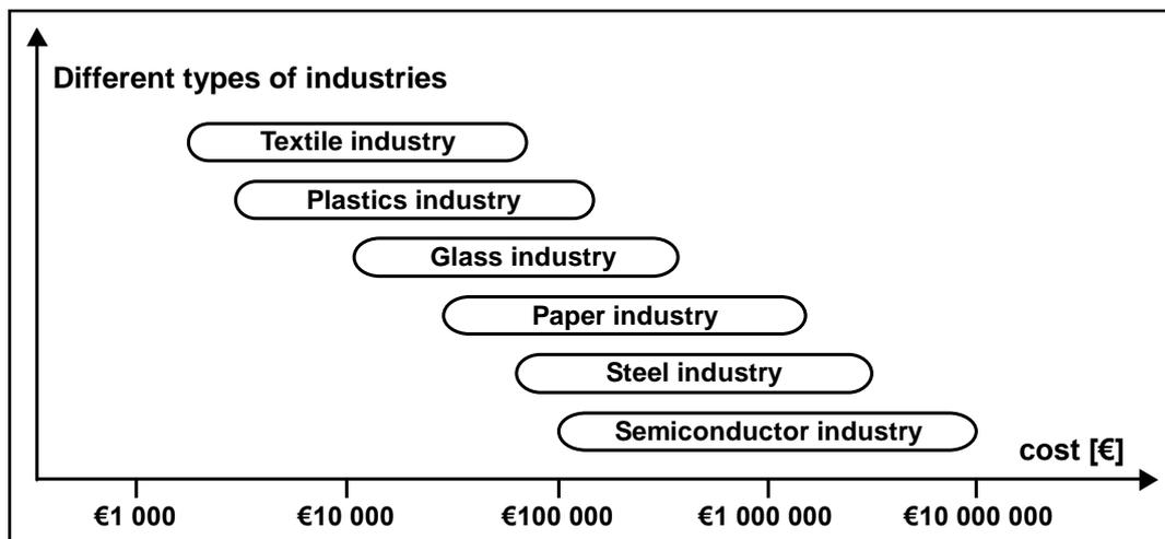
Figure 5 – Sensitivity of voltage dips to different industries, STRI AB and Vatenfall, 2002.
