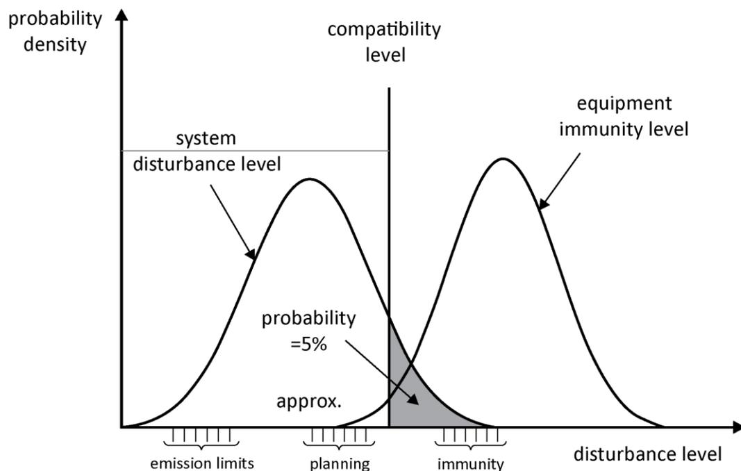
Figure 1 – Relation between compatibility, immunity, planning and emission levels according to IEC 61000-2-12.
