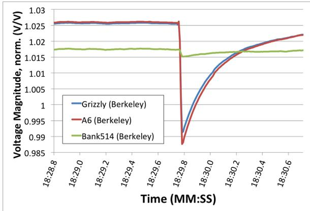
(c) Voltage magnitudes (L3 phase) measured by  $\mu$ PMU devices on different feeders in Berkeley: Grizzly and A6 on the same feeder, and Bank514 on a separate feeder. Normalized to bus nominal voltages.
