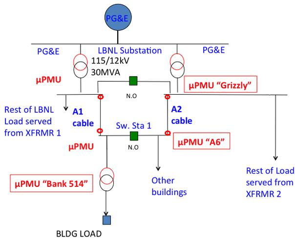
Fig. 1: LBNL  $\mu$ PMU deployment map (simplified)
